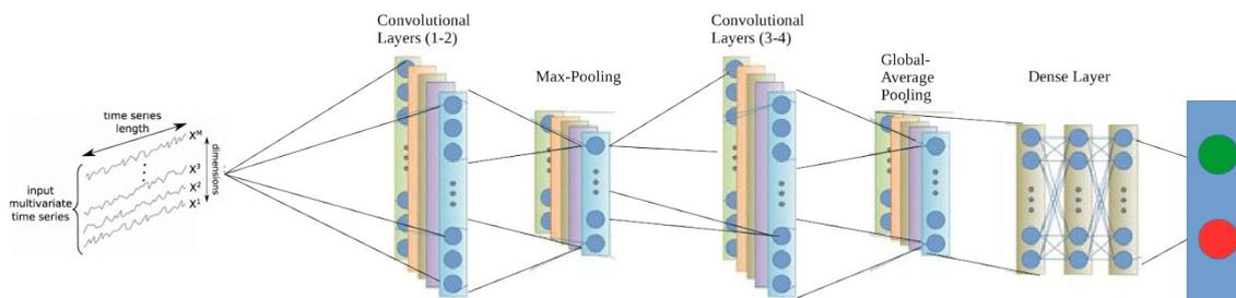
**Figure 2:** A schematic representation of MTS-CNN. It is composed of an input layer followed by two convolutional layers (1-2), a Max-Pooling layer, followed by two additional convolutional layers (3-4). Finally, a Global Average Pooling layer and a Dense layer finalizes the architecture.
